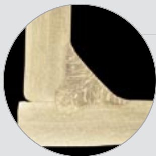
Inomaxx® Plus MAG fillet weld in 6mm thick AISI 316L stainless steel
