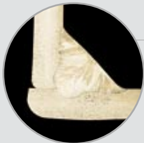
Inomaxx® 2 MAG fillet weld in 3mm thick AISI 316L stainless steel
