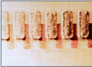
Offset printing of solder paste on printed circuit board pads.
