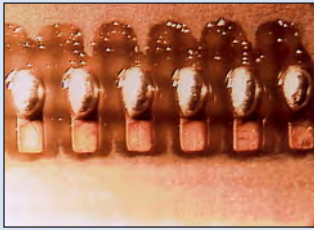
Reflowed in air atmosphere, poor wetting and high concentration of flux residue.
