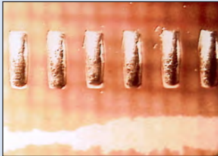
Reflowed in nitrogen atmosphere, excellent wetting and minimal to no flux residue.
