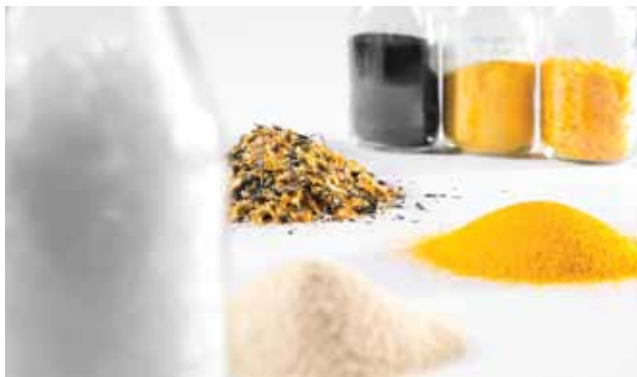
▲ Figure 2. Liquid nitrogen is used in certain particle-size-reduction processes to super-refrigerate material, including pigments, plastics, powder coatings, waxes, pharmaceuticals, nutraceuticals, spices, and other food products. Liquid nitrogen makes a material more brittle, allowing it to be easily broken up into small particles using less energy.
